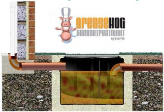
Grease Hog Grease Treatment range features 2 Grease Traps which come with an option of Standard FG range or FGH Filtered models as shown above. Catering from a nominal capacity of 170 litres in the model 1 units to 450 litres in the model 2 units. They will store/trap 100 litres and 350 litres of grease respectively.
